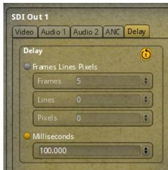
This enables the user to delay SDI output based on either frame/line/pixel values or absolute millisecond values.
