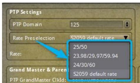
The Rate Preselection menu allows the user to define timing behavior according to the desired video frame rates. Options such as 25/50, 23.98/29.97/59.94, 24/30/60, and S2059 default rate reflect common broadcast standards. It also allows the device to align its internal timing to match those used in an environment.
