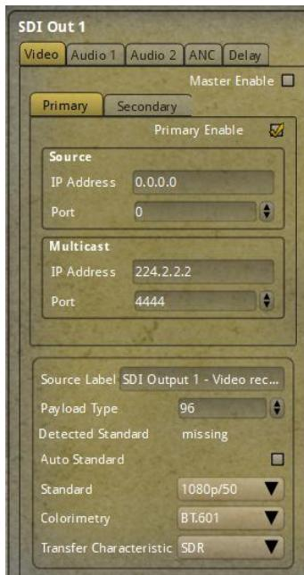
The user can control conversion from ST 2110 IP streams to physical SDI outputs (SDI Out 1 and SDI Out 2). Multicast IP and port fields are configured to receive streams. Payload type, detected standard, and manual override for video format (e.g., 1080p/50), colorimetry (BT.601, BT.2020), and transfer characteristic are configurable per output.
