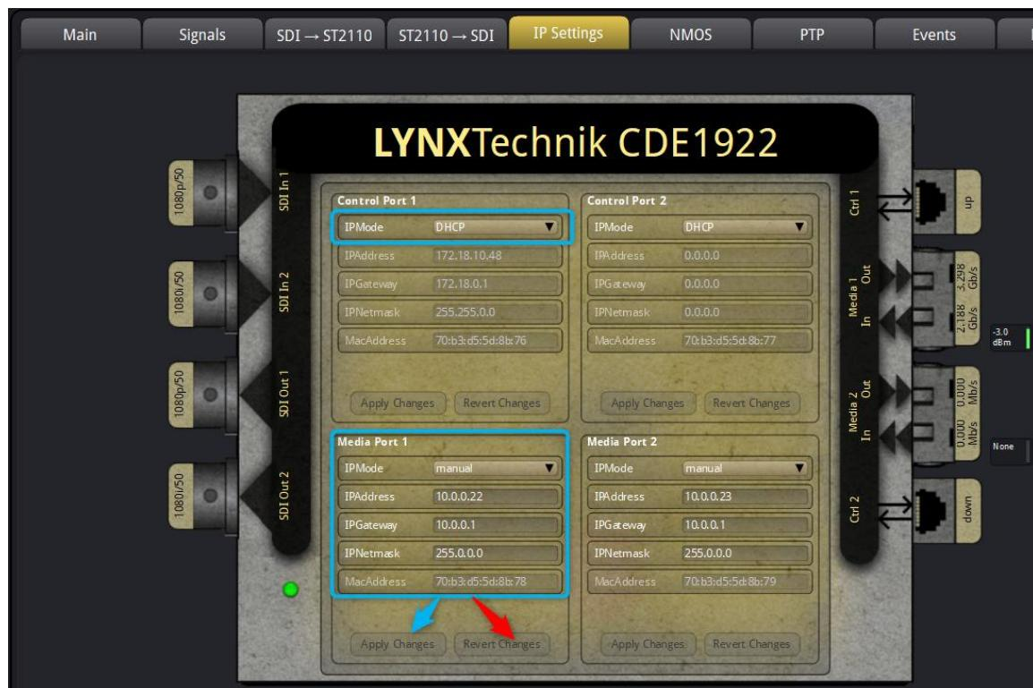
Both Media Port 1 and Media Port 2 can be manually configured, which is often preferred in deterministic production environments to maintain strict multicast routing and consistency. Media Port 1 and 2 can be set to identical gateway and subnet mask settings. Configuration changes can be staged and then either applied or reverted, giving the user control over pending modifications.
