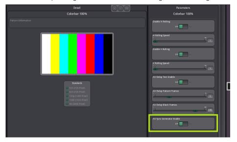
The greenMachine will now overlay the AV Sync Overlay to the test signal fill the audio channels automatically with the different dinus tones.
