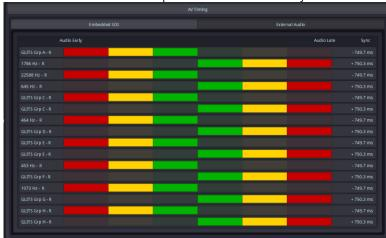
The "Sync" column will provide the audio delay measurement in ms. Delayed audio will have a measurement in +ms and early audio will have a measurement in -ms.
