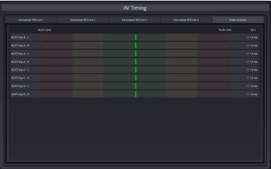
The external audio page will provide AV sync information of 8 external Analog/digital audio channels.
