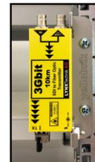
The optional RFR 1000-1 rack mount can be used to permanently mount up to 14 yellobrik modules. One or two RPS 1001-1 power supplies should be ordered separately to provide primary and optional redundant power to all modules mounted in the rackframe.
