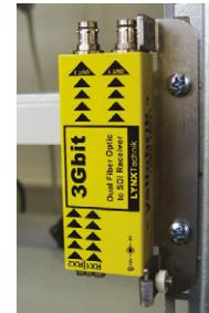
The optional RFR 1000-1 rack mount can be used to permanently mount up to 14 yellowbrik modules. In addition, the RFR 1000-1 can provide full power redundancy for all mounted yellowbriks.
