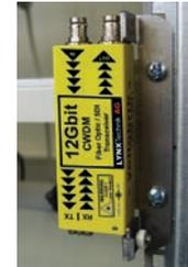
The optional RFR 1000-1 rack mount can be used to mount up to 14 yellobrik modules permanently. In addition, the RFR 1000-1 can provide full power redundancy for all mounted yellobriks.
