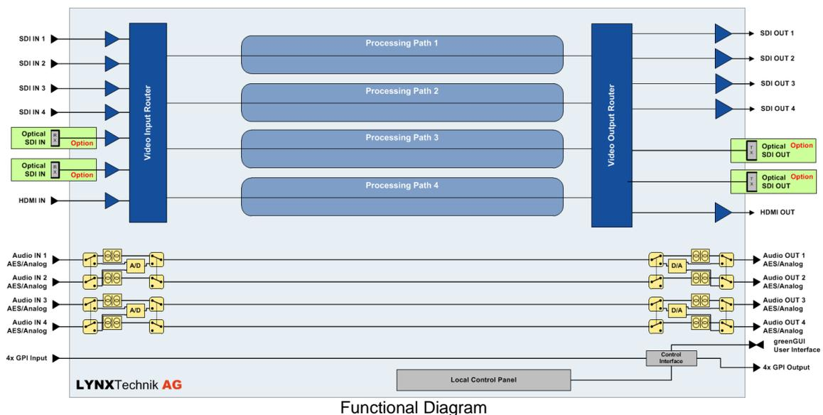
Alternatively, the greenMachine titan can be configured with one 12G capable Processing Path.
