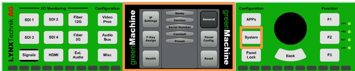
*Note: The areas on the left and right side of the display show the active menu items. Turning the rotary push encoder will navigate between these different menu items. The inverted menu item (i.e. dark gray with white text) is currently selected.*
