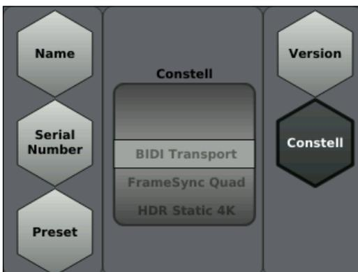
*Note: The hexagon shaped items are parameters. When one of these menu items is selected, the middle area of the display will show the type of parameter and the current setting.*
