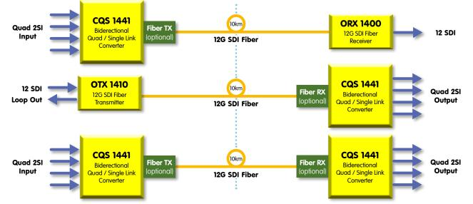
A fiber Transceiver option is also available. This includes both a Transmitter and Receiver in a single SFP package. The receive and transmit functions cannot be used simultaneously, but this option is useful if the CQS 1441 configuration is frequently changed where fiber transmission is sometimes needed and on other occasions fiber reception.
