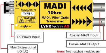
Note: Two matched modules are supplied. "A" version is shown. "B" version connections are identical.
