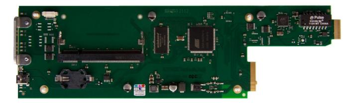
The R CT 5023 is the basic controller card and is all you need to connect a Series 5000 2RU rack frame to the APPolo Control software. The controller card has a LAN network interface that uses the LAN connection on the terminal plate of the rack frame. All LAN related settings are stored on an internal flash memory. Each controller card in one system needs to have an individual IP-address.
