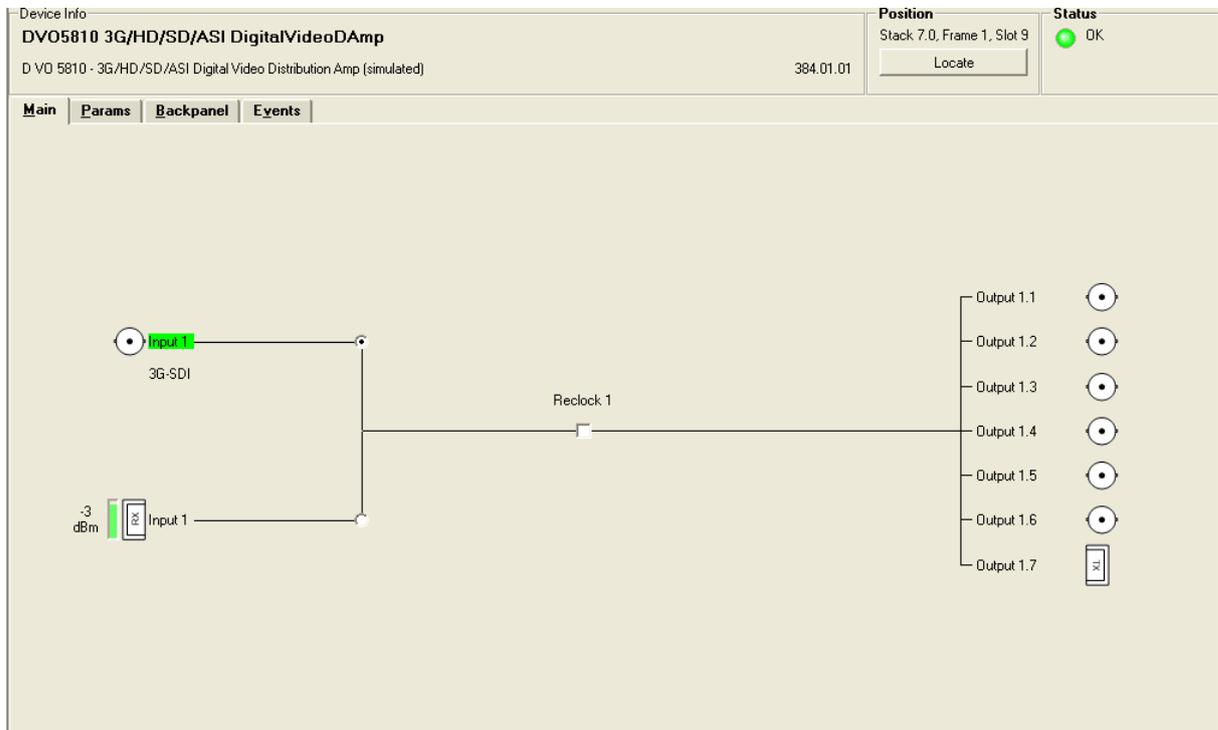
The input detection indicates the bit rate (SD-SDI = 270MBit/s, HD-SDI = 1.5 GBit/S; 3G-SDI = 3GBit/s) of a connected signal. If no signal is detected the color of the input detection will turn red.
