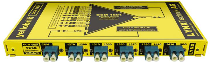
The **OCM 1891** is a compact CWDM passive 9 channel optical multiplexer / demultiplexer designed to send or receive up to 9 individual signals over a single fiber link. The module has an UPG (Upgrade) port to connect to the OCM 1892, which expands the capability of the modules to 18 CWDM channels
