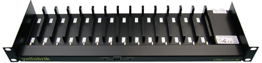
The RFR 1000 is a compact 1 RU high mounting frame designed for yellobriks. Up to 14 yellobriks can be vertically mounted and are mechanically clamped securely in place. Each slot has its own integrated power connector on a central power bus.
