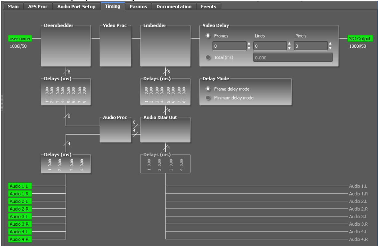
The video delay ( up to 62 frames) can be adjusted either in frames, lines and pixels or in ms.
