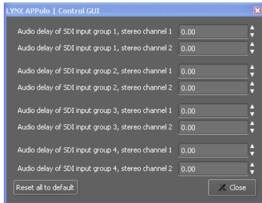
Adjusting the Audio delay in any of these locations is the only way to adjust the relative timing between Video and Audio (i.e. lip-sync corrections). Audio timing controls are offered in the context of the input as well as the output. This helps to eliminate a dependency on the routing crossbars, while you are adjusting audio-timing.
