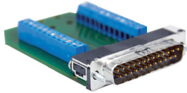
25 Pin SubD Adapter PCB with screw terminals
