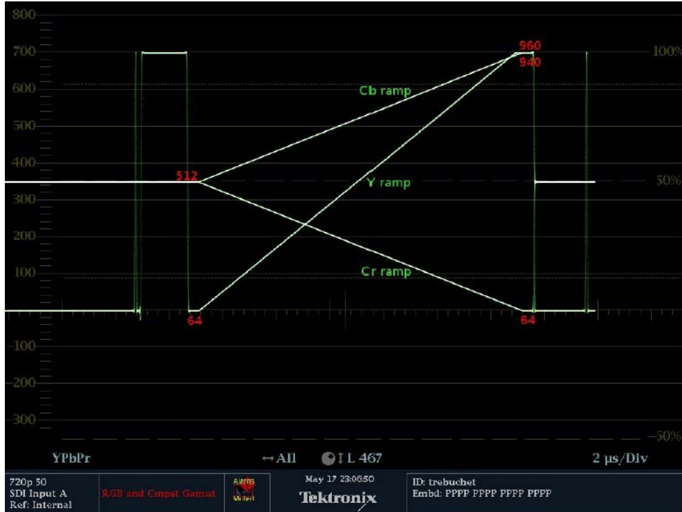
Fig 4. Y,Cr,Cb ramp for HDTV modes of operation
