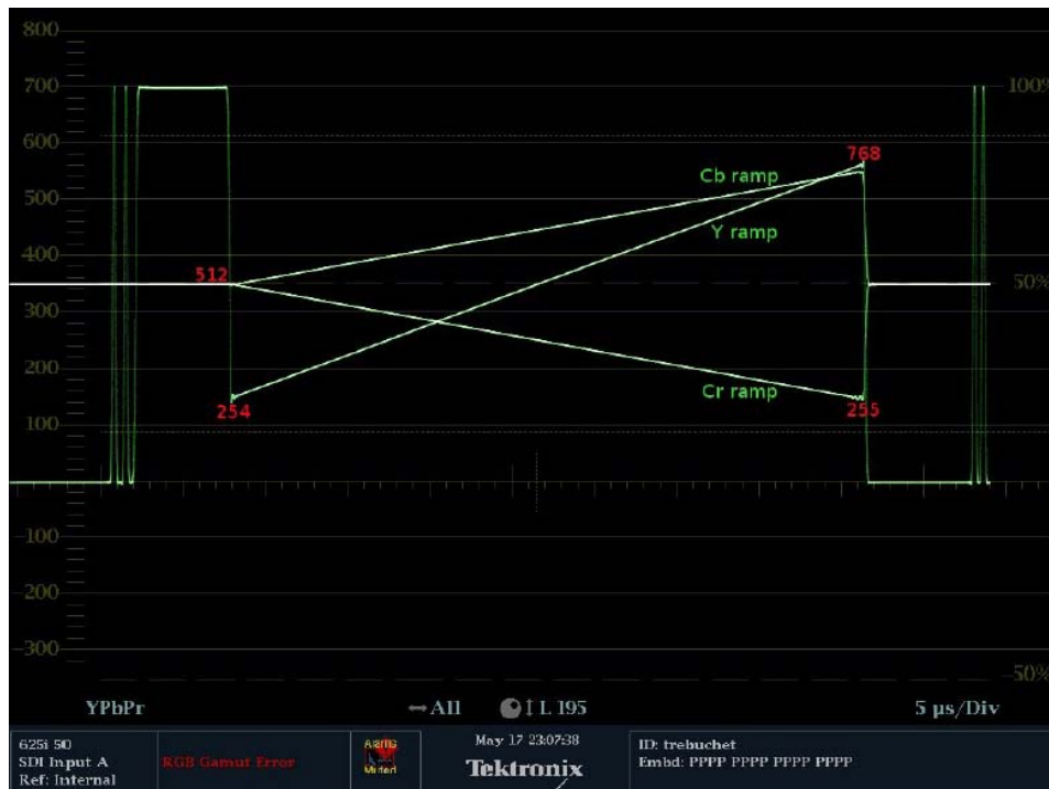
Fig 3. Y,Cr,Cb ramp for 525 and 625 modes of operation
