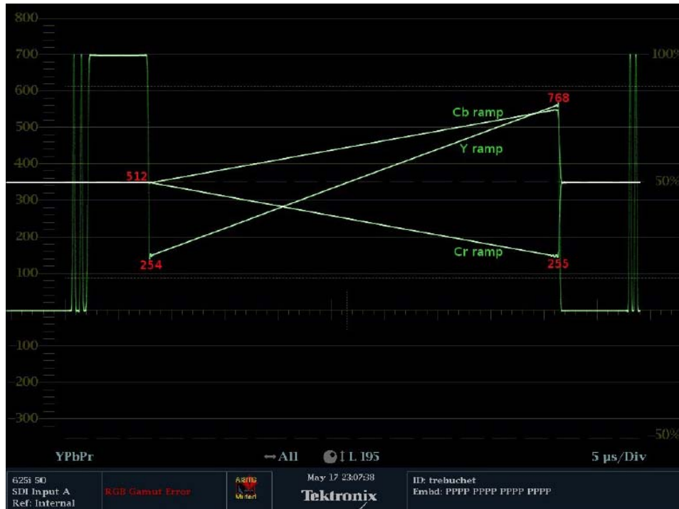
Fig 3. Y,Cr,Cb ramp for 525 and 625 modes of operation
