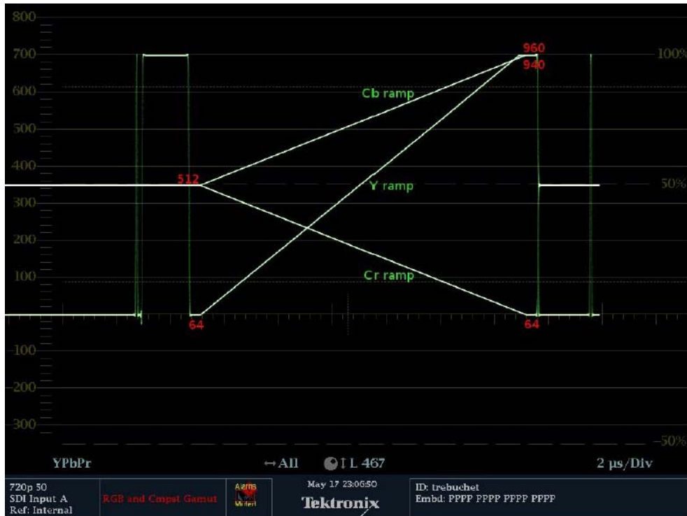
Fig 4. Y,Cr,Cb ramp for HDTV modes of operation
